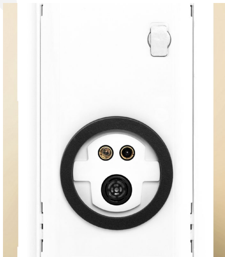
The underside of the GT 1230, with integrated cargo sensor and tamper detection seal.
