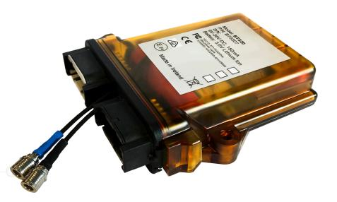
The BT 320 delivers an extensive temperature, reefer fuel and maintenance management solution for refrigerated vehicles with two-way reefer controls, temperature compliance data, accurate location tracking, EBS connectivity and real-time alerts. Integrated with FleetManager, the BT 320 allows customers to continuously monitor and maintain the integrity of temperature-sensitive cargo out on the road.
